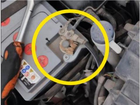
A photograph showing a close-up of a battery terminal. A pair of orange-handled pliers is being used to disconnect a metal terminal from a post. A yellow circle highlights the terminal and the pliers. The battery is grey and has various warning labels. |
