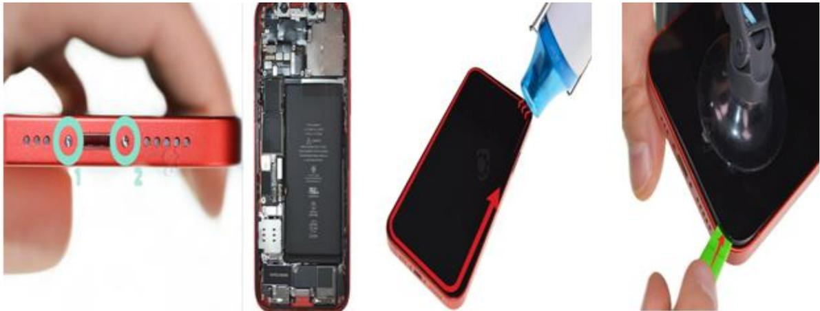
Figure 15: retirer le dos du Smartphone.
