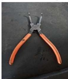
Figure 33: Pince circlips
