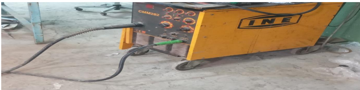
Figure 25:soudage MIG MAG
