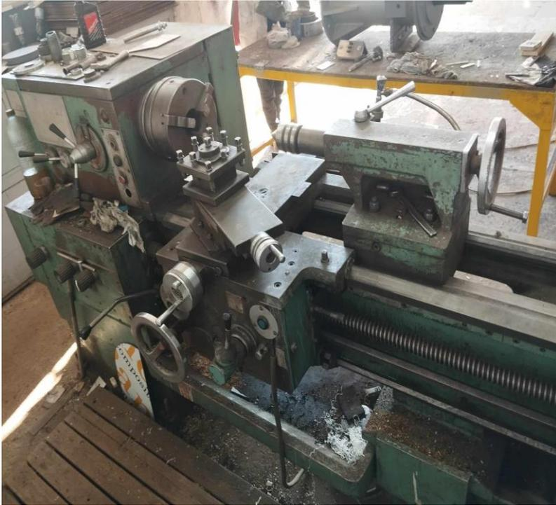
Figure 23: Machine de tournage
